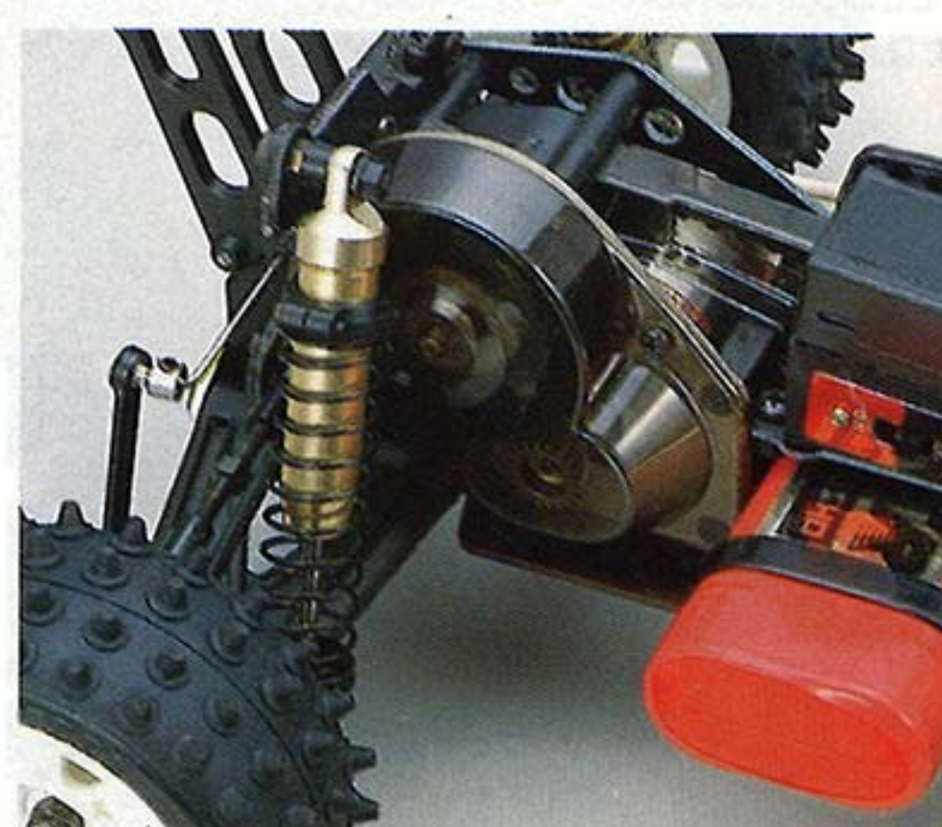
INTERNAL TORQUE LIMITER PREVENTS MOTOR DAMAGE IF WHEELS JAM.
